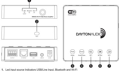
2. WPS Button for network connection and factory reset
