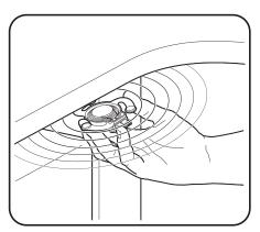
NOTE: Before permanently attaching the Sound Exciters, test the placement for optimal sound reproduction.
